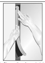
1. Clean all surfaces in joint area to remove loose debris, dirt, oil, wax, grease, old caulking, etc.
