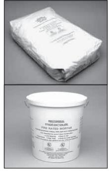
Adhesion to Cables Good Freeze-Thaw Resistance Excellent Workable Pot Life Approximately 45 minutes Sets hard 3 - 4 hours Fully Cured 28 days Yield 2.1 mix ratio 1500 cubic inches per 45 lb bag 3:1 mix ratio 1350 cubic inches per 45 lb bag
